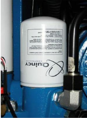
The initial filter change should occur after the first 500 hours of operation. During normal service, the filter cartridge should be replaced under the following conditions, **whichever occurs first**:
