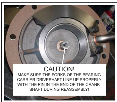
Fig. 5-5 Driveshaft Alignment
